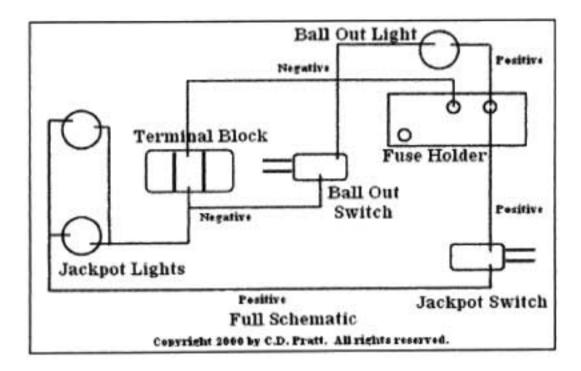
Don't forget. A lamp must have both a positive and negative current to light up.
