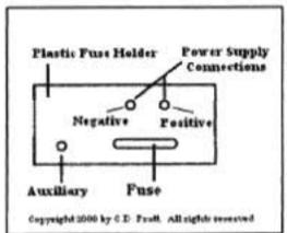
Looking at the back of the Fuse Box Holder you'll be able to tell what color wires are connected to the positive pin and which to the negative pin. Now you know what color carries positive current for your machine, and which color carries negative current.
